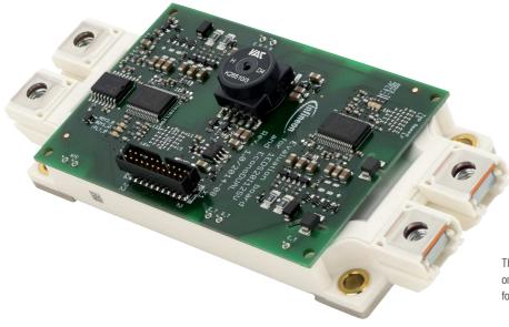
The new gate drive transformer T60403-F5046-X100 on Infineon's evaluation board EVAL-1EDS20I12SV for the EconoDUAL<sup>TM</sup> 3 IGBT series
