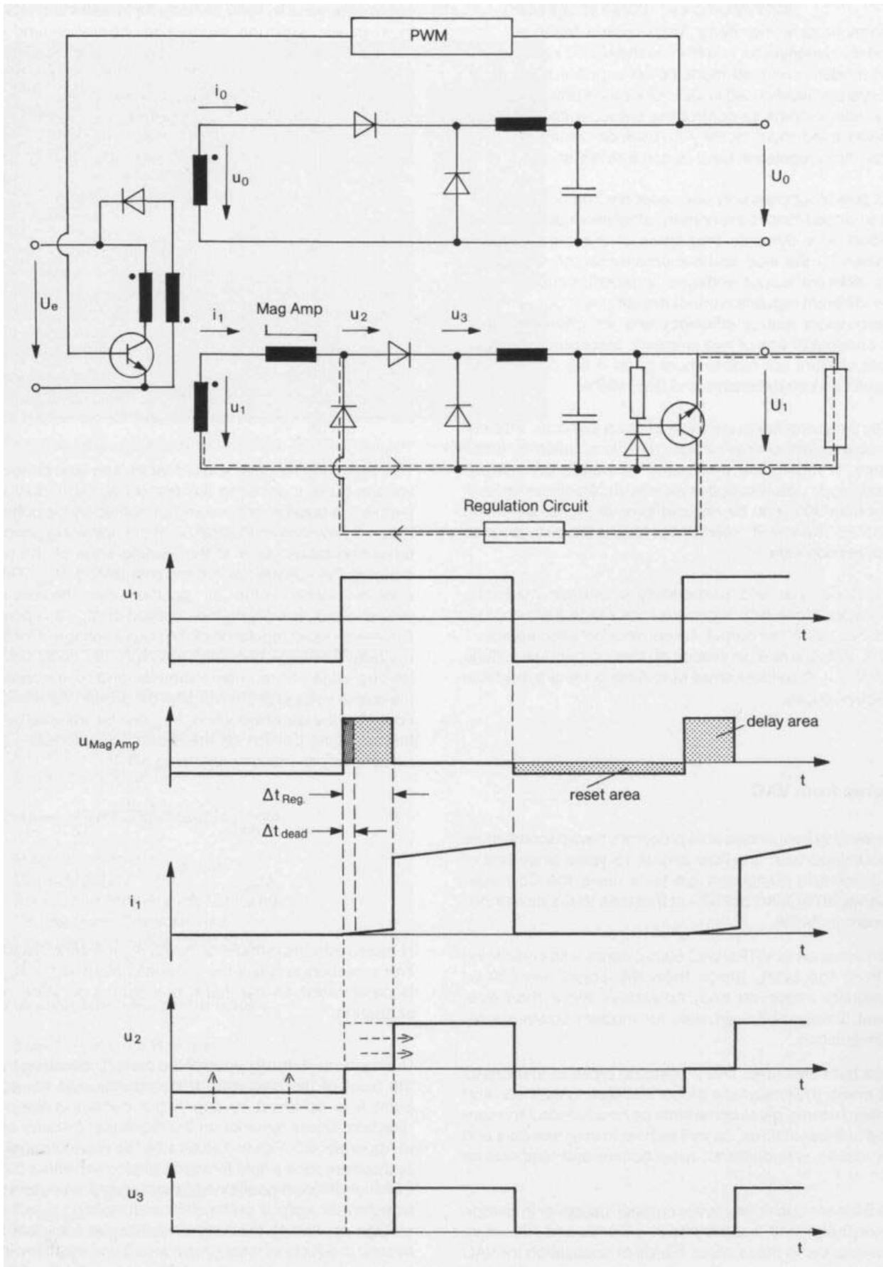
Figure 1: Basic Operating Principle of Magnetic Amplifier Regulation
