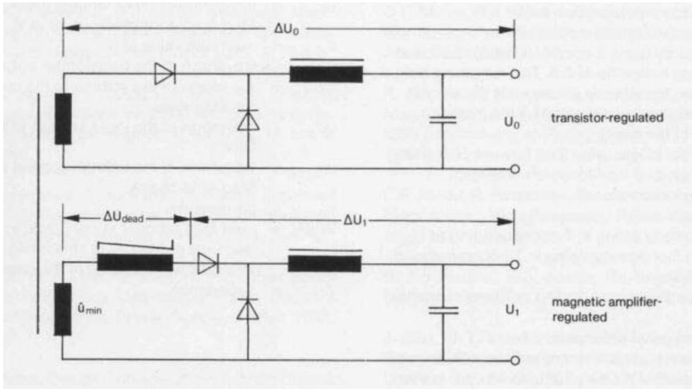
Figure 7: Principle Circuit with Voltages and Voltage Drops
