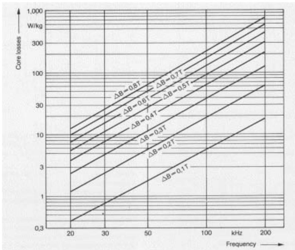
Figure 3: Typical Core Losses of VITROVAC 6025 Z Cores
