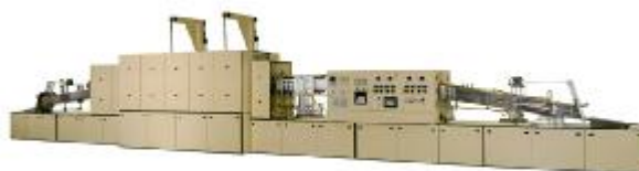
Figure 1: Controlled atmosphere conveyer belt furnace (Tokyo Braze)
